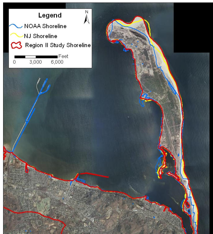
Figure 4. Extracted (red), best-available NOAA shoreline (blue - 1974), and NJ State shoreline (yellow - 2002) compared to 2008 aerial photograph at Sandy Hook, NJ.
