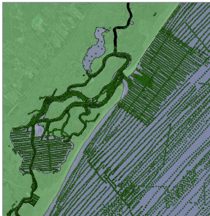
Figure 14. Feature-class components of the bathymetric TIN or ESRI Terrain.
