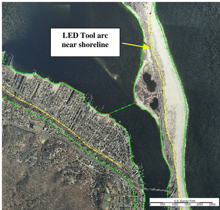
Figure 33. Example of nearby feature determining the spacing along LED Tool feature arc
