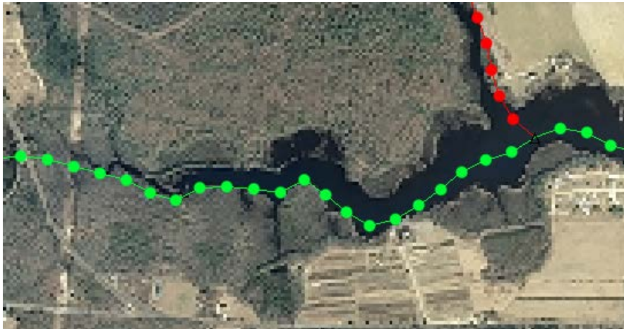
Figure 14. Alternative solution for a narrow stream with only one feature arc, with nodes placed on one side of the river
