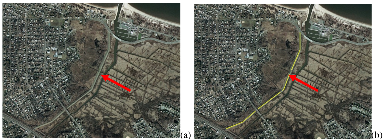
Figure 32. Example of (a) a ridge feature that could serve as a flow barrier and (b) the ridge as detected by the LED Tool
