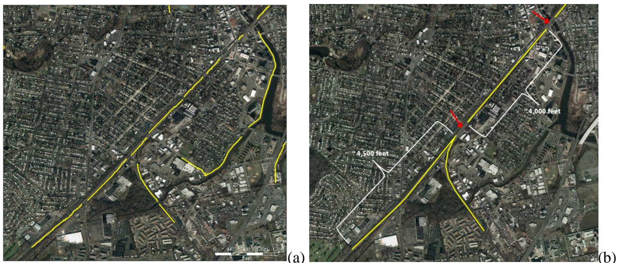
Figure 48. Sample area where (a) multiple LED arcs are (b) combined to result in fewer gaps with longer LED arcs
