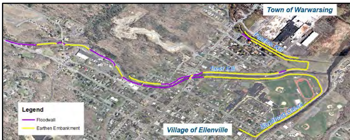
Figure 2: Levee Embankments and Floodwalls
