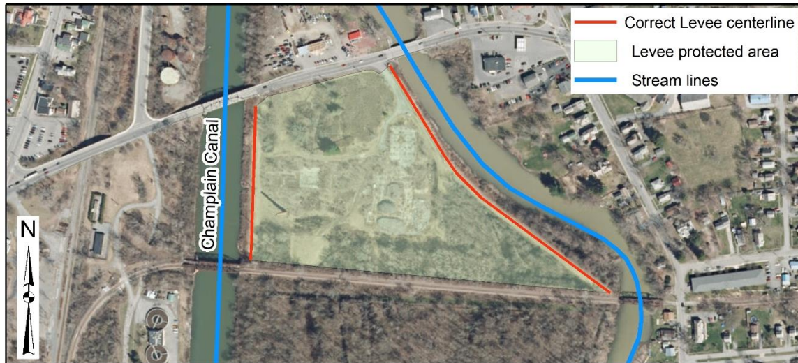
Figure 2: Correct levee centerline
